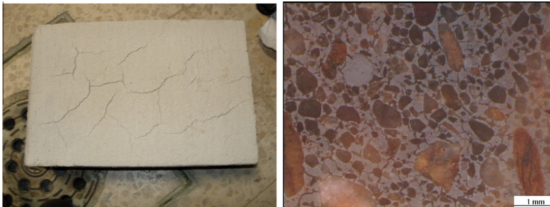
Fig. 5. Mortar prepared with quicklime pieces, QM.1-7 (7-day maturation).
