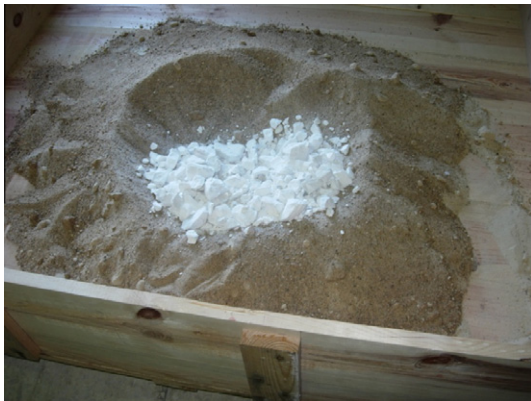
Fig. 4. Introduction of the quicklime into the sand mix.
