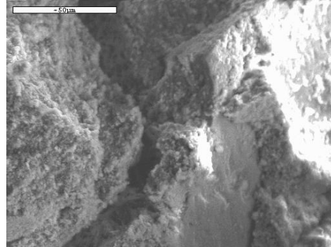
Fig. 4 Tc, dense mortar microstructure and internal cracking in the lime matrix
