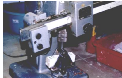
Fig. 3 Testing of flexural strength
