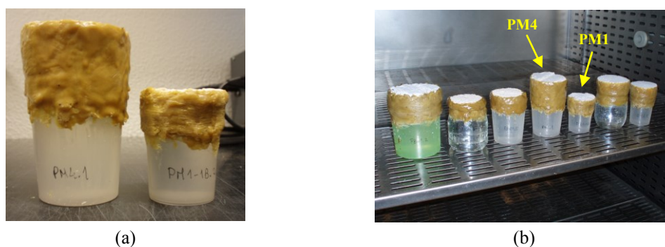
Figure 4.91 - Water vapour permeability determination in samples PM1 and PM4: (a) devices used (adapted to ancient samples); (b) ongoing test
