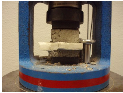
Figure 4.104 - Adapted compressive strength test: ISF3 “sandwiched” between two layers of confinement mortar
