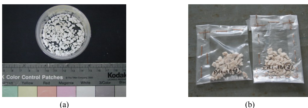
Figure 4.9 - Preparation of the test specimens for mercury intrusion porosimetry: (a) sample EG4 (thin-layer plaster) before drying; (b) sample PM1 ready to be tested
