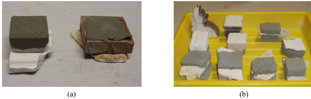
Figure 4.13 - Adaptation of ancient plaster samples to the compressive strength test device: (a) application of the shaping mortar; (b) samples ready to be tested
