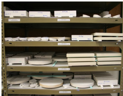
Figure 5.2 - Storage of the test specimens in conditioned environment
