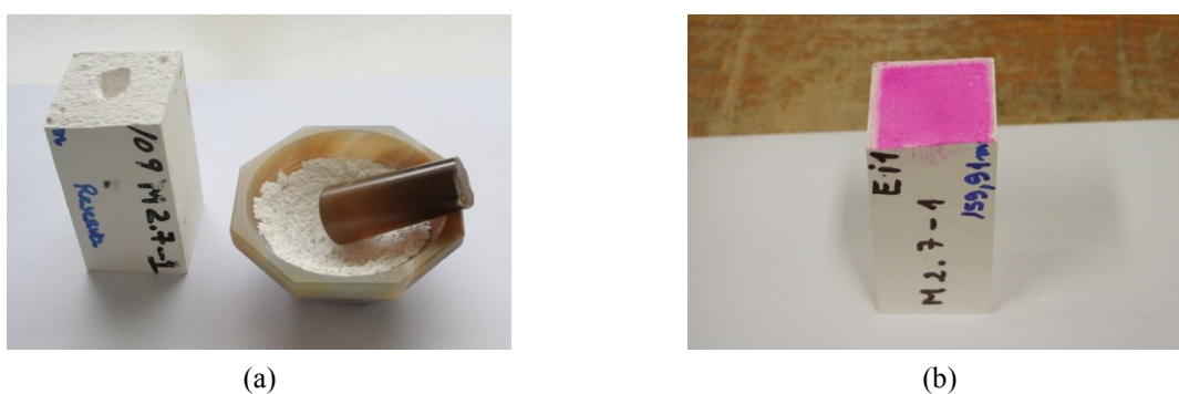
Figure 5.18 - Evaluation of the carbonation process: (a) preparation of samples for TG-DTA analysis; (b) surface of a test specimen a few seconds after being sprayed with phenolphthalein
