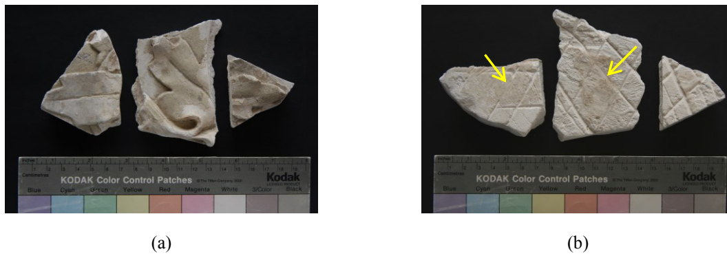
Figure 4.78 - Sample PM2: (a) front view; (b) back view, with synthetic film (yellow arrows)
