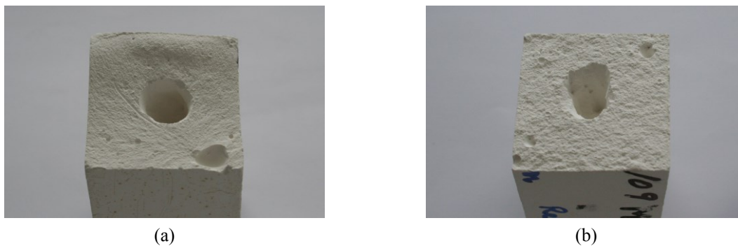
Figure 5.25 - Surfaces of test specimens after failure showing textural differences: (a) L1; (b) M2
