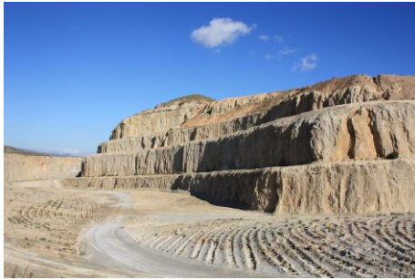
Figure 2.1 - Gypsum natural deposits: (a) open quarry in Almeria, Spain, with very thick gypsum beds ( http://www.panoramio.com/ ); (b) thin layer of satin spar gypsum embedded in a clayed ground ( http://academic.emporia.edu/aberjame/student/corley3/rdhil.htm ); [accessed 15 September 2015]
