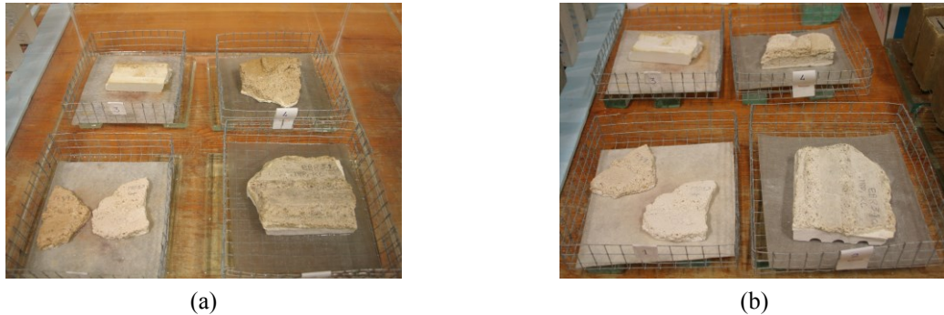
Figure 4.5 - Determination of the capillary water absorption in ancient samples using a contact technique: (a) samples in a vat where water reaches the bottom of the baskets (absorption procedure); (b) baskets placed in stands outside the vat (drying procedure)
