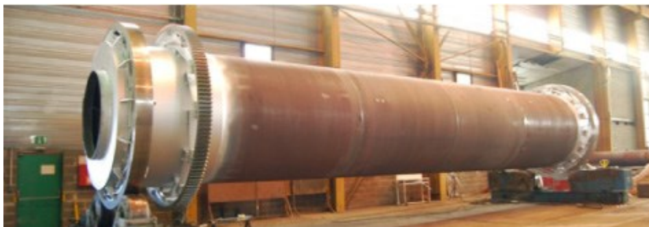
Figure 2.11 - Directly fired rotary kiln used to produce \beta -hemihydrate and multiphase plasters
