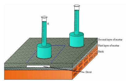
Figure 7: Brick samples water absorption test scheme. Application of Karsten pipes in areas only with base mortar and in areas with grout under base mortar (g).
