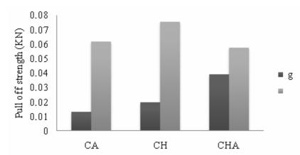
Figure 9: Results from pull off strength tests on brick samples (Darker bars represent values from areas with grout (g) and brighter grey bars represent areas without the grout).
