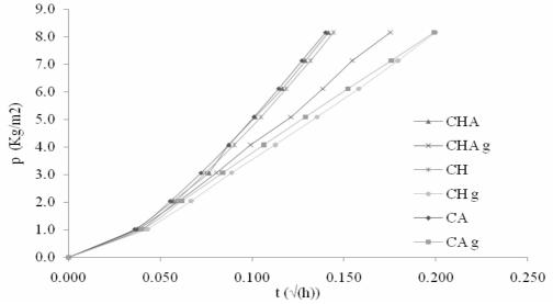
Figure 8 – Water absorption, with time, behavior for the different compositions.
