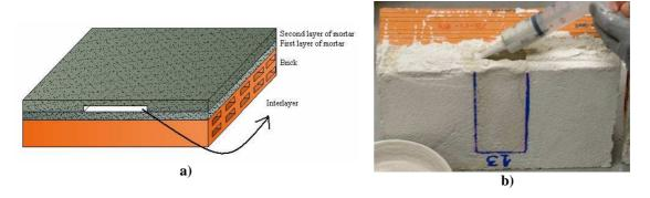
Figure 2: a) Brick samples scheme; b) Grout application on a brick sample
