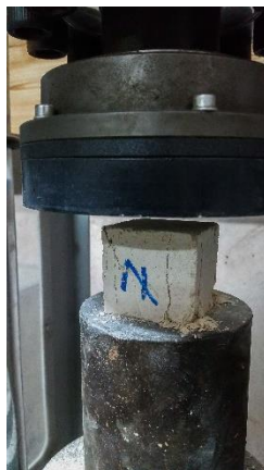
Fig.3: Compression test setup
