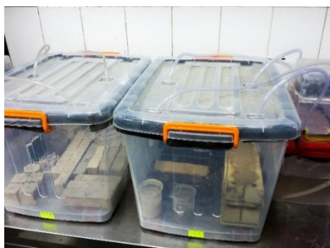
Fig.1: The controlled environmental chamber
