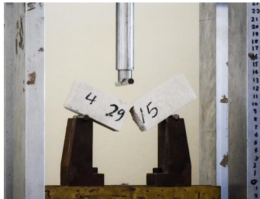
Fig.10: Flexural strength test setup
