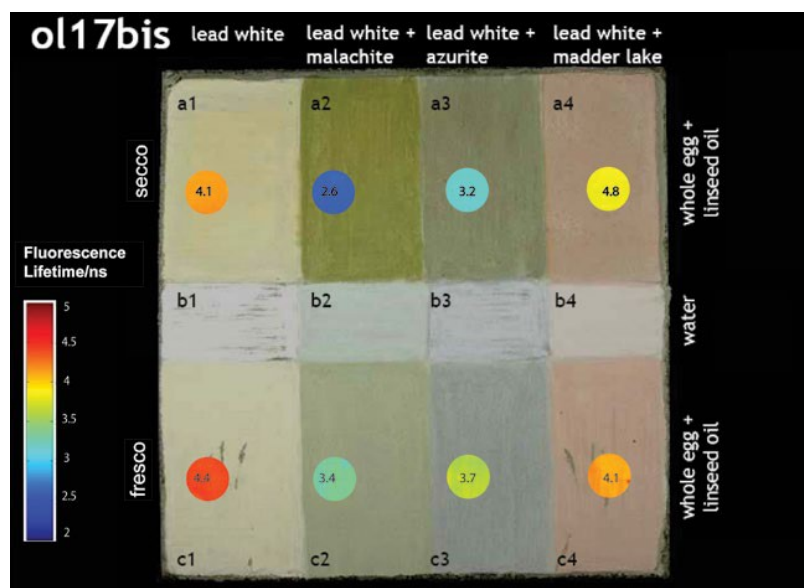
FIGURE 7 False-color FLIM of replica OL17b. The colors of the circles represent different lifetimes.
