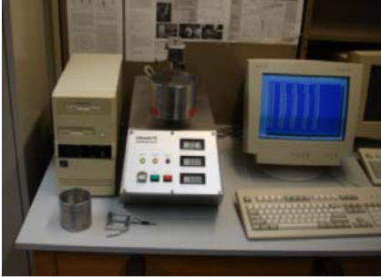
Fig. 5 – Viskomat PC rheometer used for determining the flow curves of the mixes.
