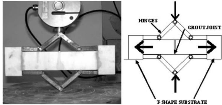
specimens was needed. As shown in Fig. 1, each composite specimen, prepared as described in Sect. 3.3, was glued (using epoxy resin) with transverse pieces of the same substrate material, to give it the form required by the applied testing method. The forces were applied by a hydraulic press (max capacity: 300 kN). A load cell (max capacity of 10 kN) was placed between the piston and the specimen; it was connected to a computer, where load measurements were transferred and stored.
