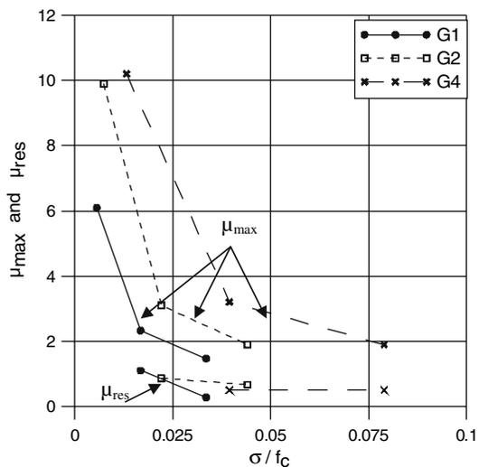
**Fig. 9** Effect of the applied normal stress-to-grout compressive strength ratio on the travertine-to-grouts friction coefficient (age 90 days)
