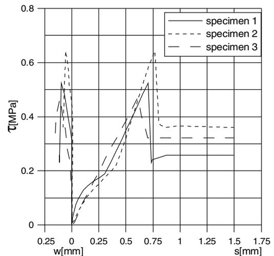
**Fig. 7** Shear stress ( $\tau$ ) versus shear slip ( $s$ ) and lateral dilatancy ( $w$ ) for marble-to-grout G2 specimens (age 90 days at  $\sigma = 0.30$  MPa)
