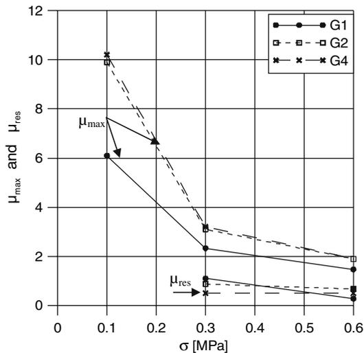
**Fig. 8** Effect of the applied normal stress on the friction coefficient along travertine-to-grout interfaces (age 90 days)
