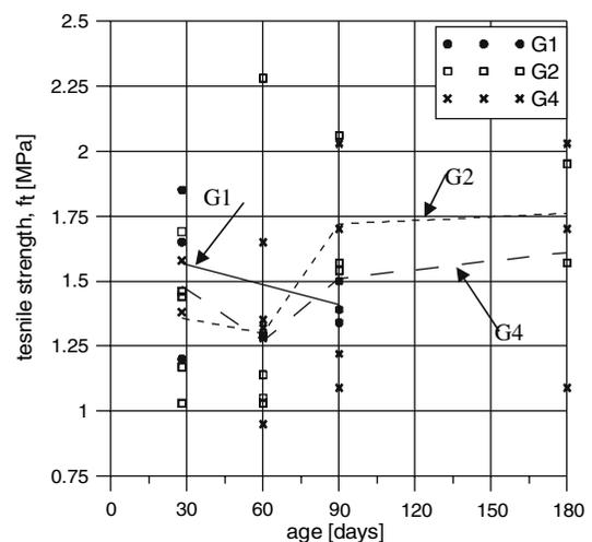
**Fig. 6** In-time development of travertine-to-grout bond tensile strength
