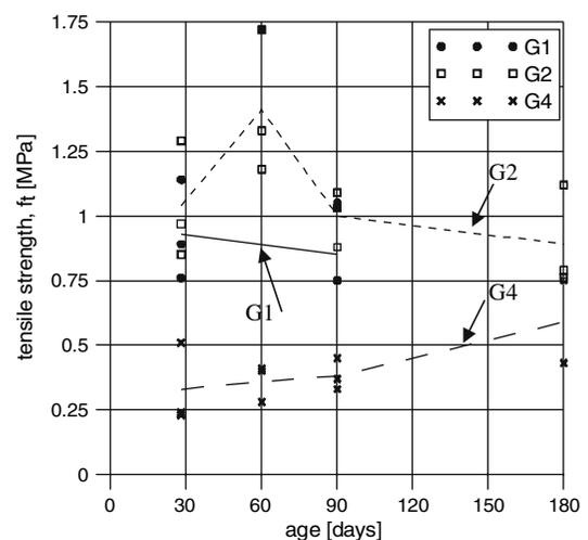
**Fig. 5** In-time development of marble-to-grout bond tensile strength
