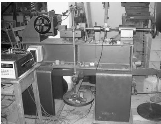
**Fig. 2** Experimental set up for shear tests
