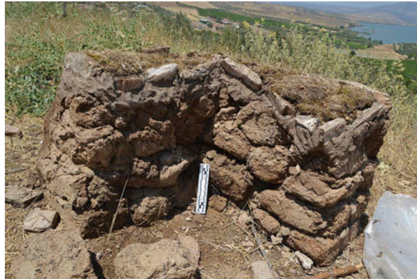
Figure 8. Soft vegetative cap applied Tekelioğlu experimental L-shaped mudbrick wall (top surface) directly after application.
