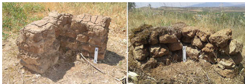
Figure 6. Tekelioğlu experimental L-shaped mudbrick wall: (a) just after construction in July 2013 (southeast side) and (b) 11 months later in June 2014 (southeast side).
