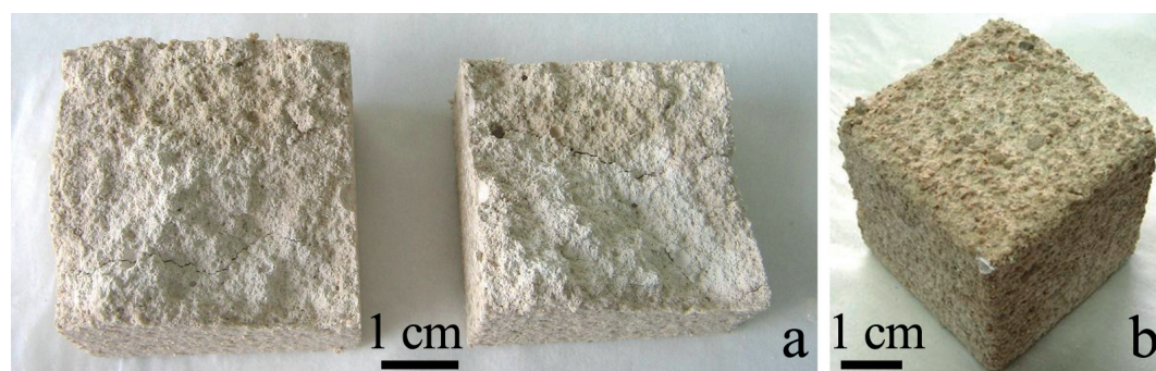
Figure 9. Broken sample with the evidence of internal fissures (a); sample after 15 cycles, showing material loss from the surface by granular disintegration (b).
