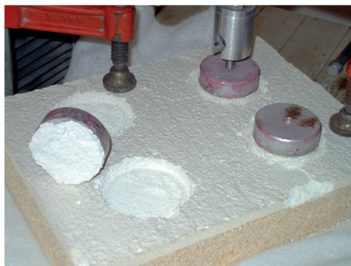
Figure 1. Adhesive strength test on the stone/mortar composite specimen.
