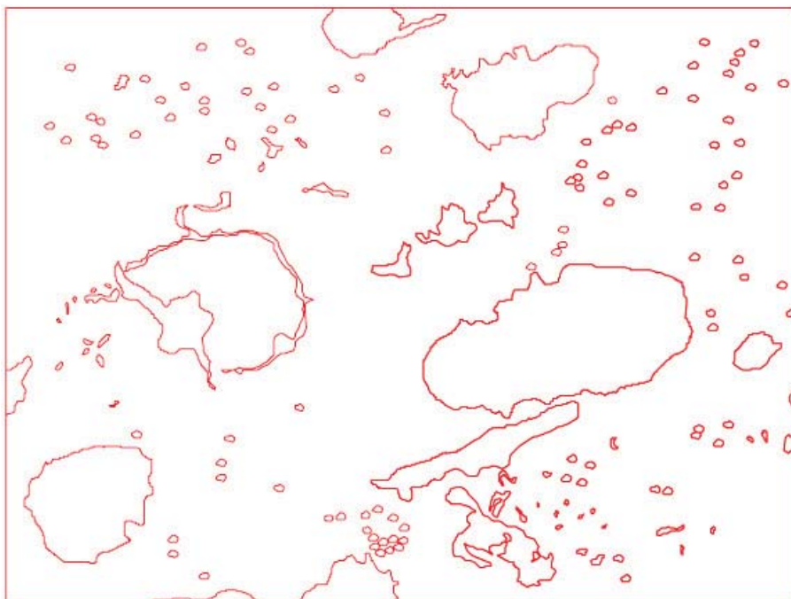
Pore Space Calculation for Burnt Puddled Earth: Sample No. 8547 Through Digital Image Analysis at 1536 x 2048 pixels
