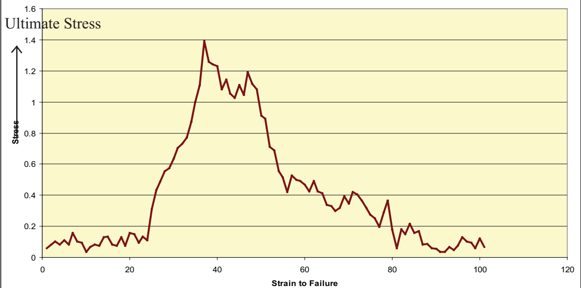
4-Point Bending Test. G.L. top=0.85", G.L. bottom=2.0". Speed=0.005 inch/min. Sample-8547
