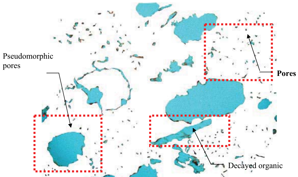
Figure 6.14: Extracted pixels of the pore spaces used for the quantitative calculation of the pseudomorphic voids to the solids
