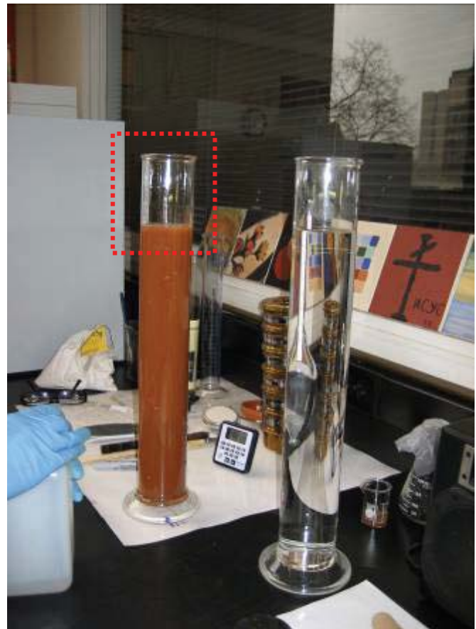
Figure 6.9: Sedimentation of Fine Particles in 1000 ml cylinders
