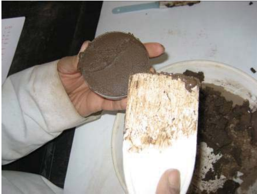
Figure 6.12: Casting the wet soil into shrinkage dishes
