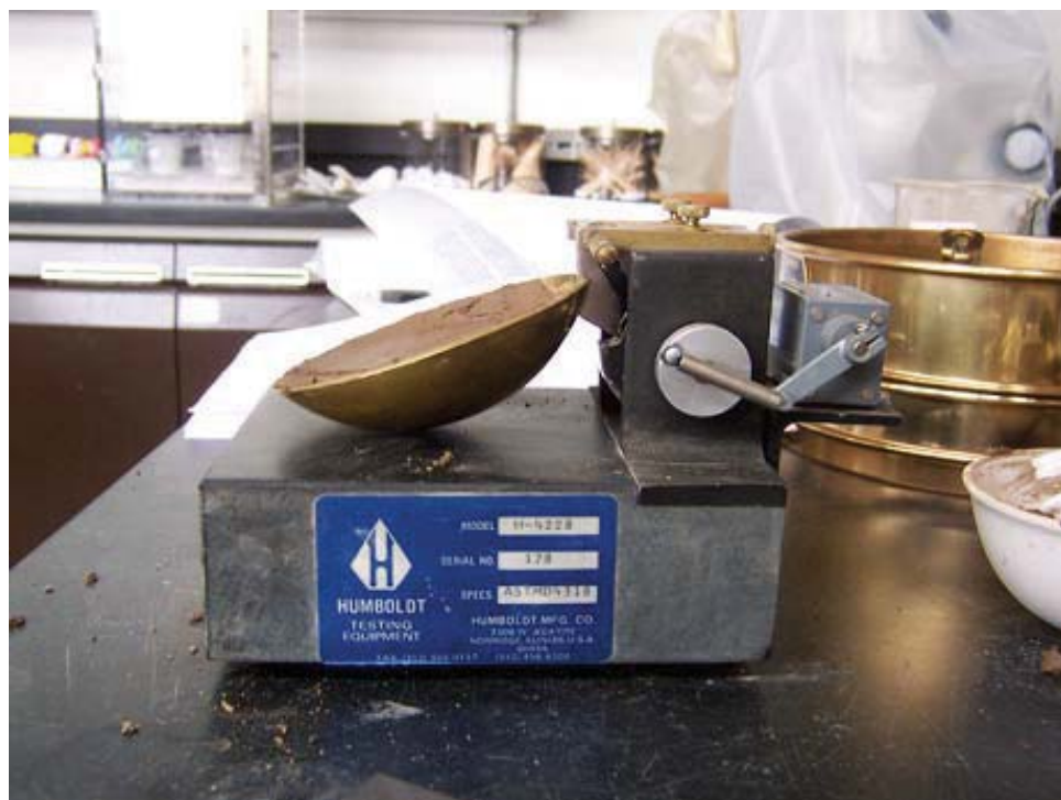
Figure 6.11: Casa Grande Device for Liquid Limit calculation
