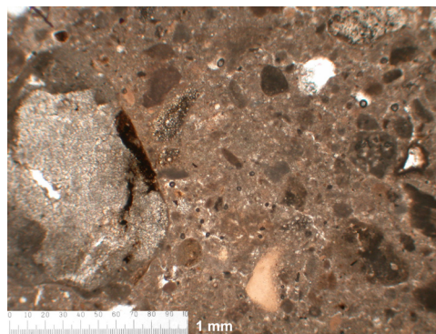
Ca23. Wall render. Early Classic. Micritic and crystalline calcite. PPL. Scale bar: 1 mm.
