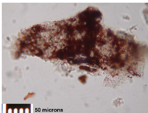
Ca5. Particle with dark red areas. Birefringence of red particles can be observed in the edges. Characterization: hematite. Left: PPL. Right: XPL. Scale bar: 50 microns.
