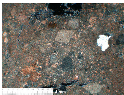
Pa49. Wall render. Otulum Phase. Hydraulic matrix, aggregates of micritic calcite and grain of quartz. Left: PPL. Right: XPL. Scale bar: 1 mm.
