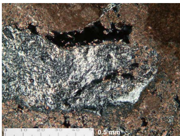
Fig. 6.12. Aggregate formed by aluminosilicate crystals, likely cordierite. Sample Ca9. XPL. Scale bar: 0.5 mm.
