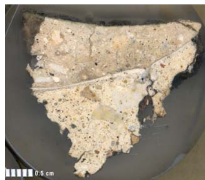
Fig. 7.24. Sample La 22 from Structure N12-12. Superimposed layers with a limewash. Macroscopic scanned view. Scale bar: 0.5 cms.
