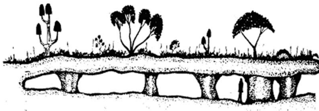
Fig. 3.3. Evidence of sascab mining with small columns left to support the limestone cap. Image: (Folan 1978).
