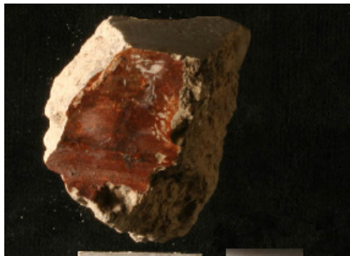
Ca5. Left: macroscopic view with red paint layer. Right: Red paint layer over limewash (hematite). RXPL. Scale bar: 0.5 mm.
