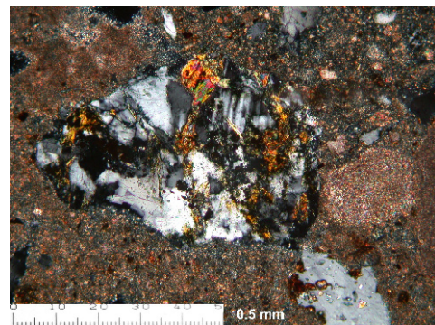
Pa53. Wall render. Balunté Phase. Rounded igneous rock with biotite mica, feldspars and opaques. Left: PPL. Right: XP. Scale bar: 0.5 mm.
