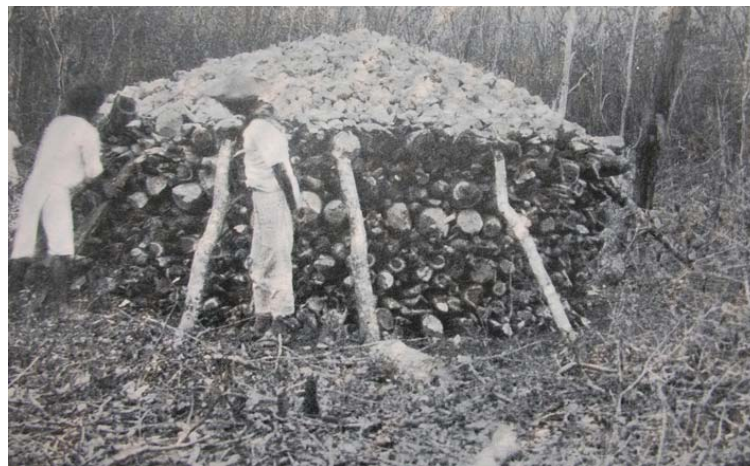
Fig. 3.5. Lime burning at Chan Kom. Picture: Refield and Villa Rojas (1934).
