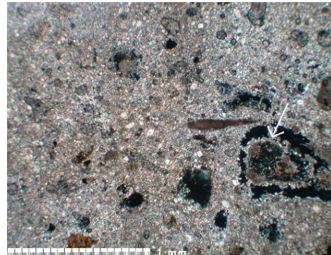
La20. Joining mortar. Early Spanish Colonial. Visible isotropic materials (likely silica gel). PPL. Scale bar: 1 mm.
