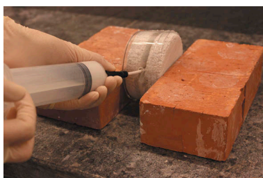
Figure 3. Injection of the grout between the two plaster slabs through the holes drilled in the plastic container.
