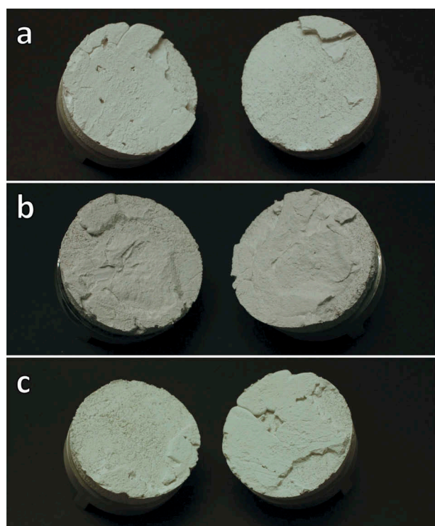
Figure 8. ‘Sandwich’ system after the adhesion test; (a) specimen S_A: the failure is at the interface between the grout and the plaster; (b) specimen S_B: the failure is in the middle of the grout; (c) specimen S_C: the failure is at the interface between the grout and the plaster; in specimen S_C the grout did not completely fill the gap between the two slabs of plaster.
