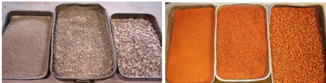
Fig. 4 Three different grain size ranges (fine, medium, coarse). Limestone sand (left picture) and Crushed brick (right picture)
