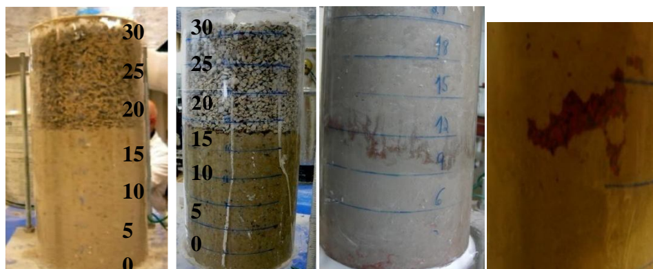
Fig. 13 Cylinders filled with media type a) D_{\text{stone,dry}} b) E_{\text{stone,dry}} c) D_{\text{brick,dry}} and d) C_{\text{brick,dry}} being injected. The flow was uniform but with different velocities of injection
