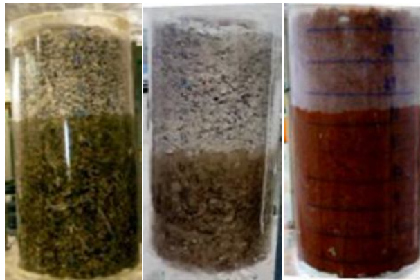
Fig. 8 Cylinders filled with media type E_{\text{stone}} (left), A_{\text{stone}} (central) and A_{\text{brick}} (right) being injected by water. The flow was uniform but with different velocities of injection
