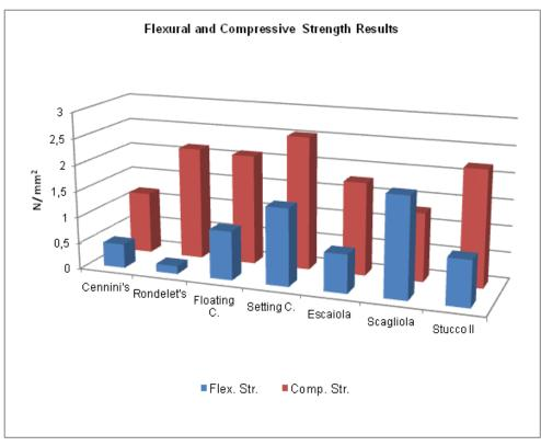
Figure 11. Flexural and compressive strength at 90 days.
