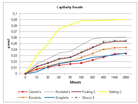
Figure 12. Capillary curves for the seven mortars at 90 days.
