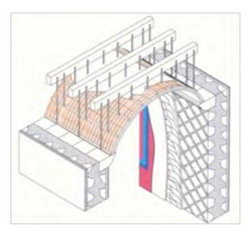
Figure 1. Roman masonry, light dome and stucco-work (Salavessa 2009).
