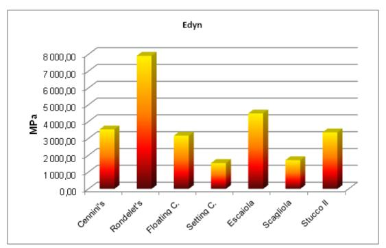
Figure 10. Dynamic modulus of elasticity at 90 days.
