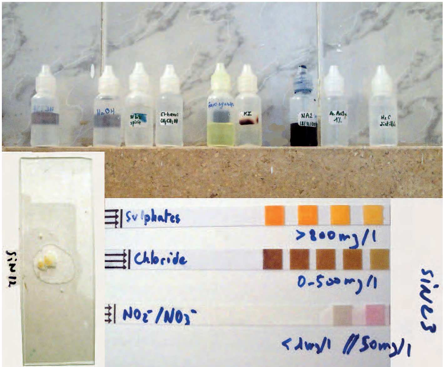
Chemical reagents (top), microchemical test (bottom, left), salt testing using chemical strips (bottom, right) on samples from Coptic wall paintings in a cave at the site of Hammâm Faraûn Sinâï (Egypt); Photos: 2010, CICRP (Jean-Marc Vallet)
