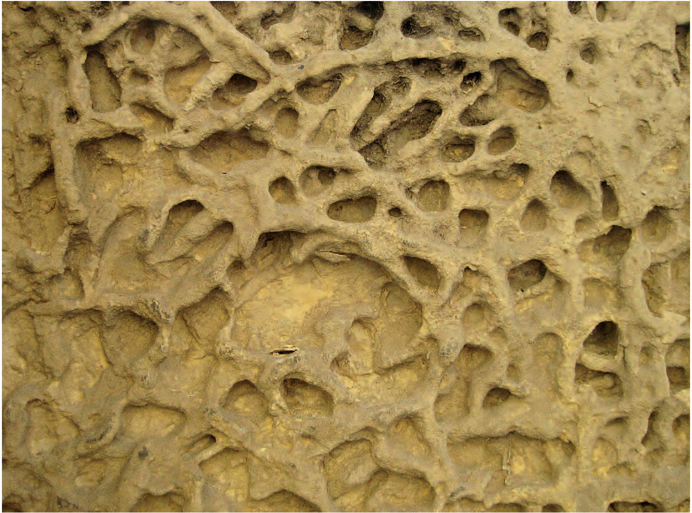
Alveolar weathering on Globigerina Limestone, due to intrinsic properties of the material (bioturbation); Photo: 2010, UM (JoAnn Cassar)
