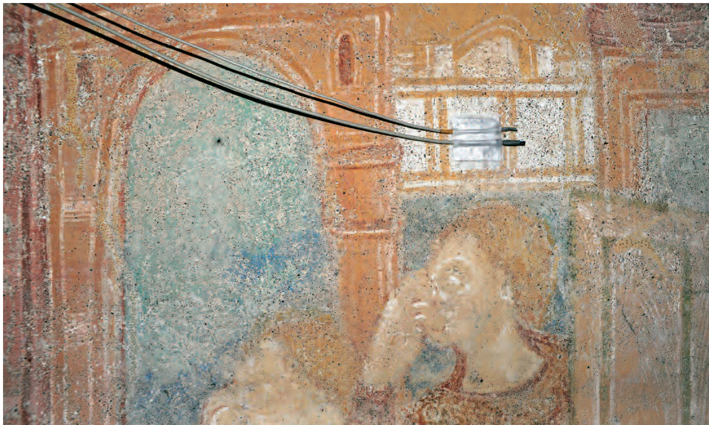
Sensors for environmental monitoring temporarily fixed with binder which sublimates (cyclododecane), St. Georg, Reichenau-Oberzell (Germany), 10th century; Photo: 2014, RPS (Dörthe Jakobs)
