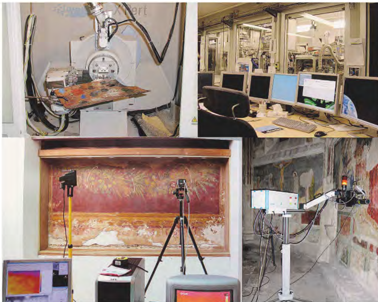
Examples of a selection of scientific methods used to analyse wall paintings in situ or samples using XRD (top, left), XANES line (ESRF, Grenoble; top, right), stimulated IR Thermography (bottom, left), \mu -XRF (bottom, right); Photos: CICRP (Jean-Marc Vallet)
