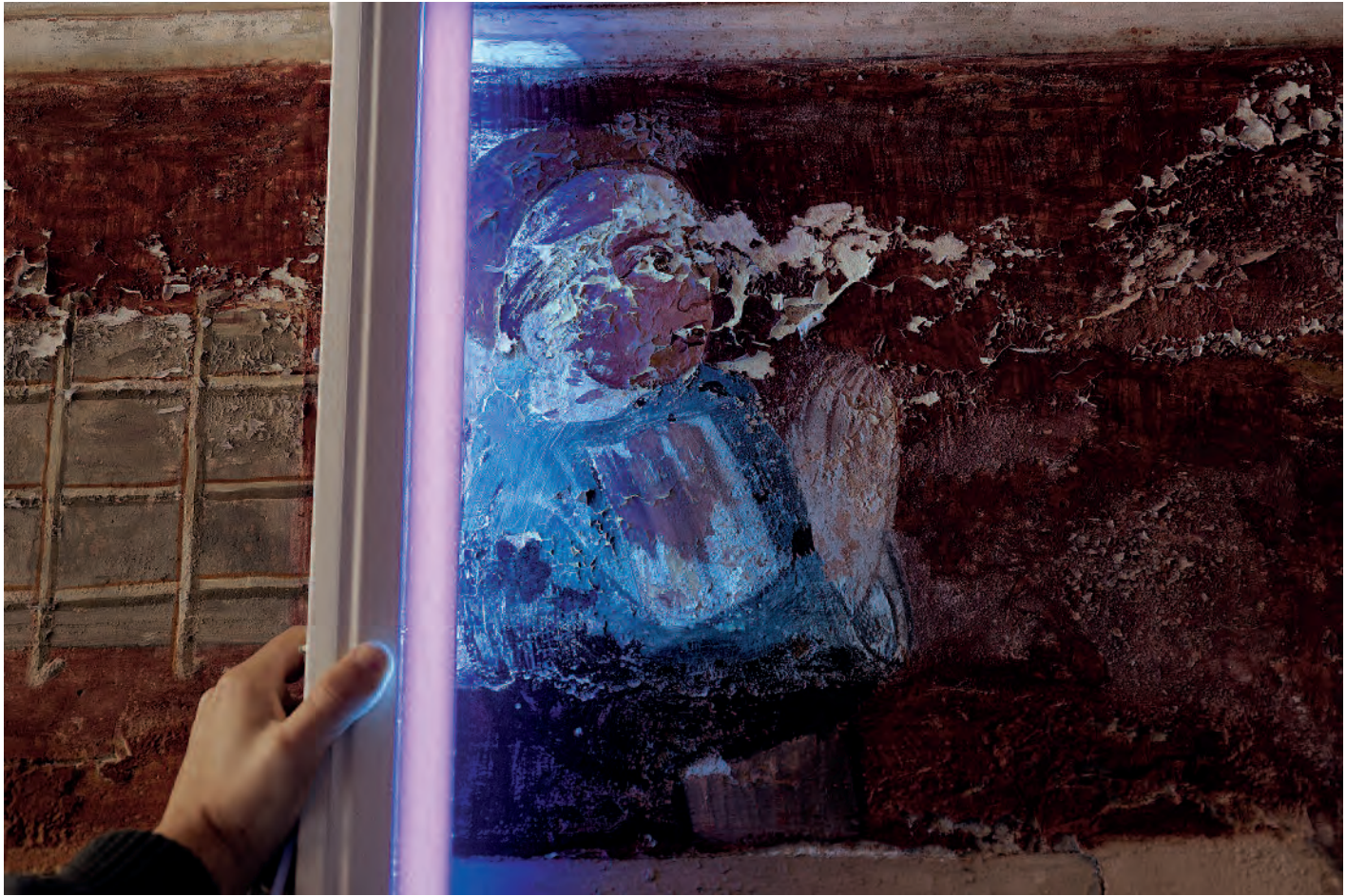
Visualisation of a restored area using UV fluorescence, Chapel of St. Sébastien, Roure (France), 15th century; Photo: 2011, CICRP (Jean-Marc Vallet)
