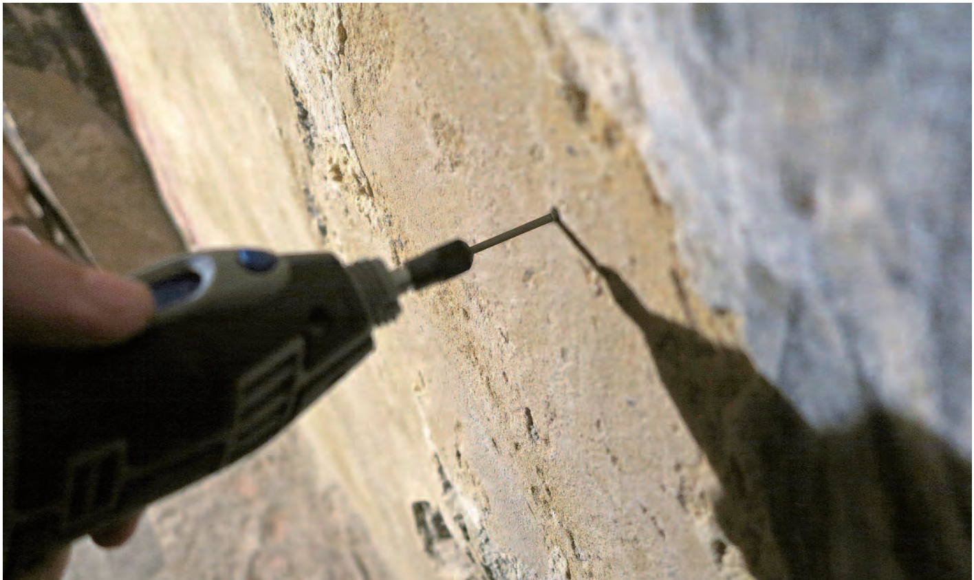
Drill core sampling of a restoration render, Chapel of Notre Dame d'Entrevignes, Sigale (France), 16th century; Photo: 2013, CICRP (Jean-Marc Vallet)
