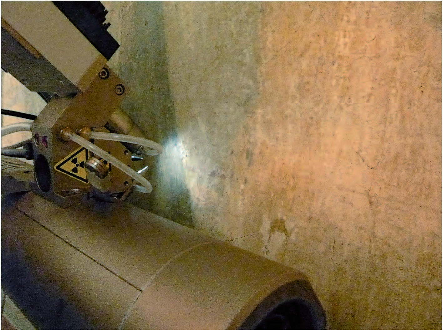
X-Ray microfluorescence measurement, detail of frescoes, chapel, Charterhouse, Villeneuve-lès-Avignon (France), 1355; Photo: 2011, CICRP (Jean-Marc Vallet)
