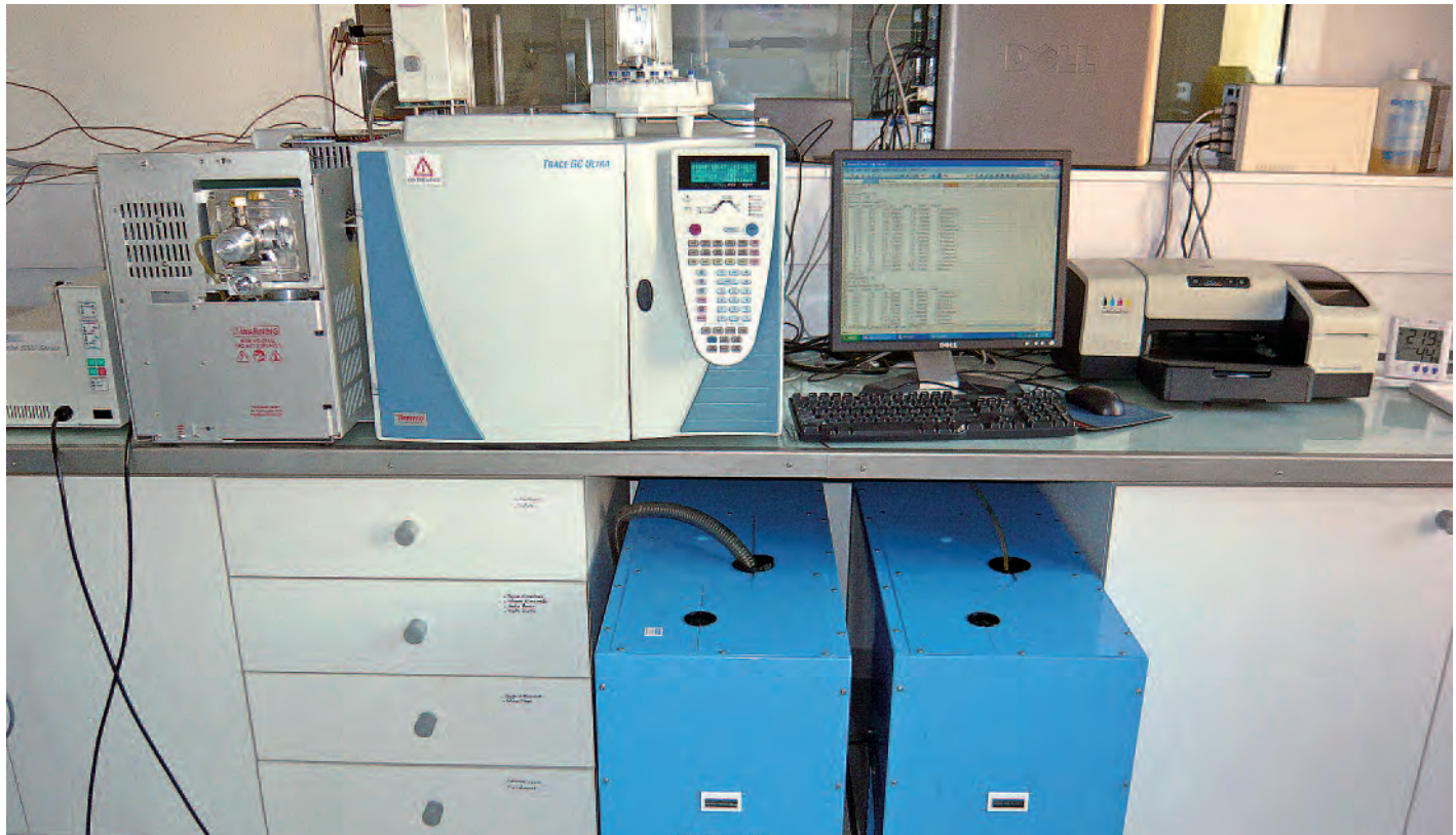
Analysis of organic binding media using gas chromatography coupled with mass spectrometry, equipped with pyrolysis; Photo: 2011, CICRP (Jean-Marc Vallet)
