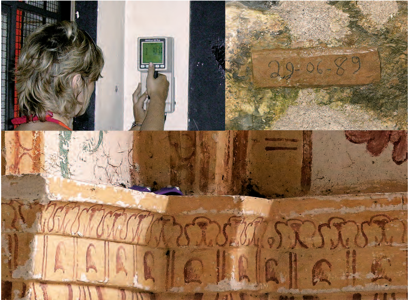
Collecting colorimetric data (top, left), crack monitor to observe deformations (top, right), Villa E-1027, Roquebrune- Cap Martin (France), 20th century and climate data logger (bottom), Chapel of Notre-Dame des Fontaines, La Brigue (France), 15th century; Photos: 2007/2014, CICRP (Jean-Marc Vallet)
