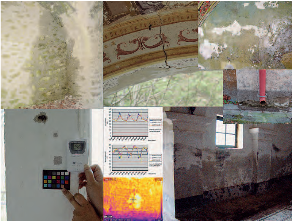
Monitoring including relative humidity and temperature measurements (bottom, left and centre) and observations including passive IR thermography (bottom, centre) relative to environmental issues; Photos: CICRP (Jean-Marc Vallet)
