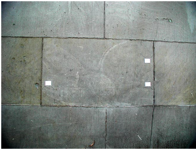
Figure 1. Labels attached for the granular disintegration test.
