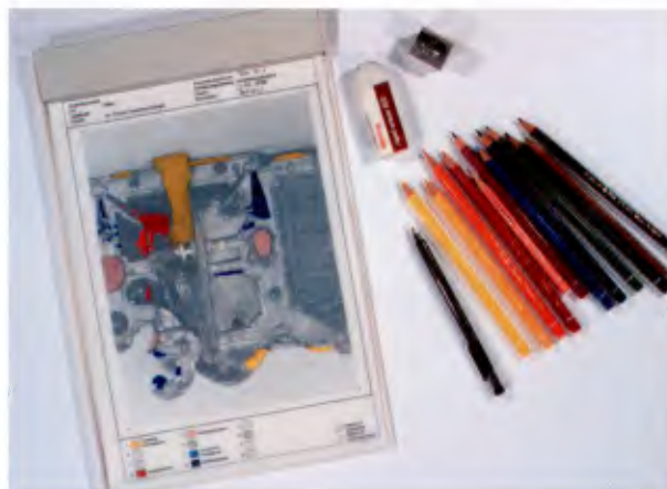
Figure 1. Materials for manual mapping. Base map and overlay are fixed congruently using a drawing board. The corners of the photographic base map are copied as reference marks on all overlays.
