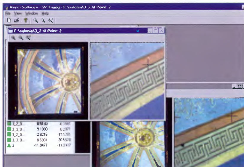
Figure 5. SV Triangulation system: This figure shows the collimation phase of the absolute orientation work phase. You have to choose homologue points on the various photos and associate them by simply clicking on them. This is one of the preliminary moments of the model creation.
