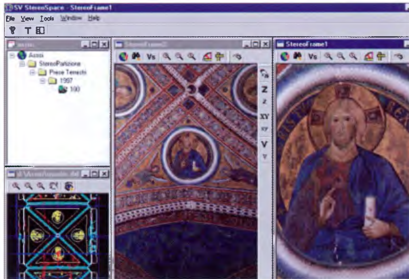
Figure 4. StereoSpace system: On the right are two opened stereo frames. Software permits opening several windows to make interesting comparisons between different zones. This feature is extremely efficient if you have two models from different time periods or showing different techniques.
