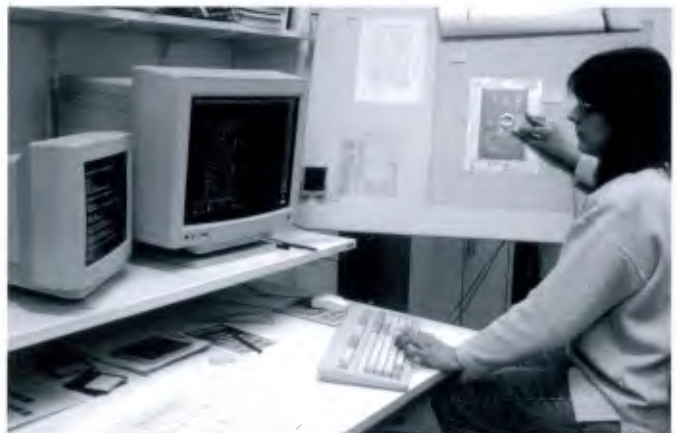
Figure 14. CAD workstation with A1 digitizer for introducing large maps.
