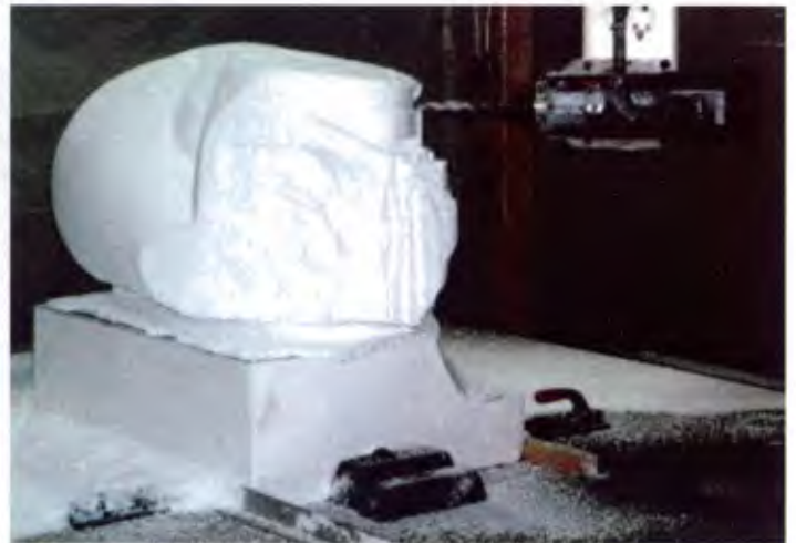
Figure 21. Leg of sculpture being carved by a milling machine at x 2.5 original size.
