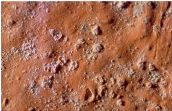
Figure 10 a/b. So-called pustules, dot-like crystallizations of salts (mostly through the formation of gypsum on the surface).
