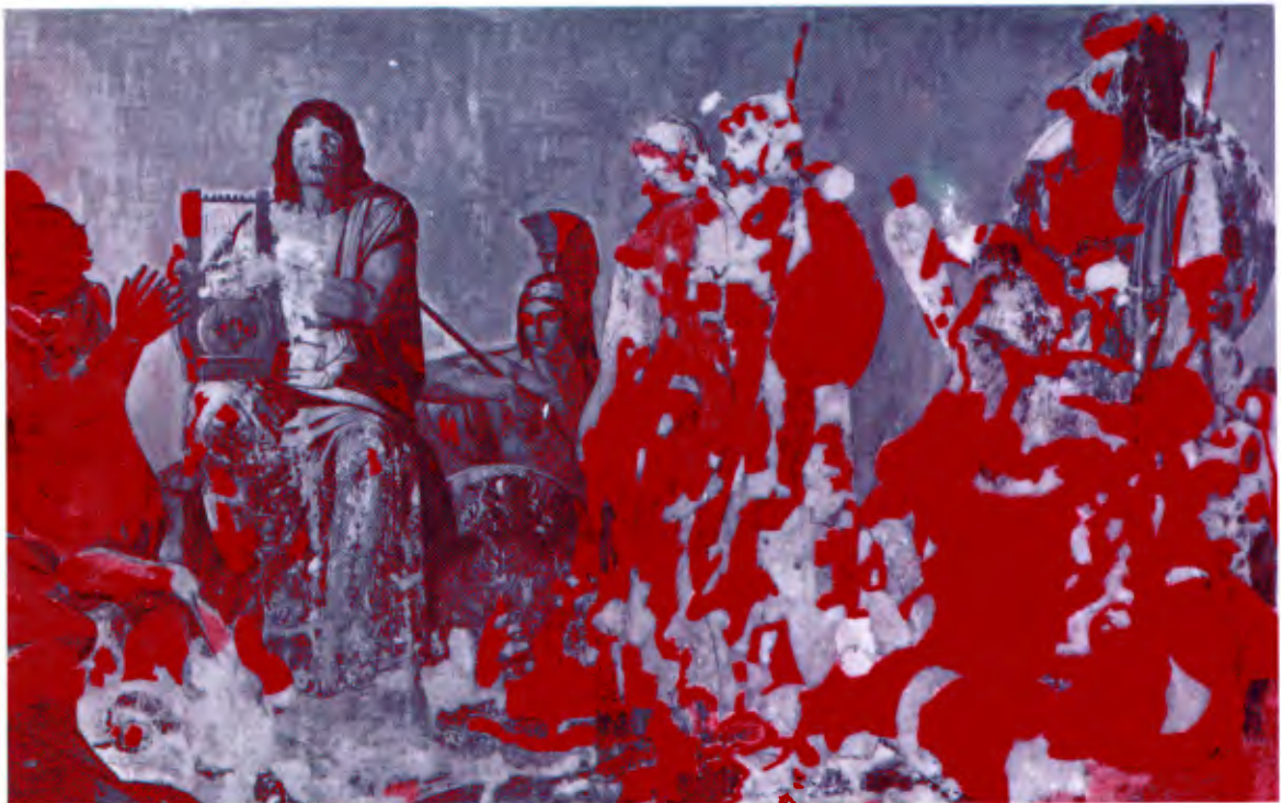
Figure 15. Munich, Ludwig-Maximilian University, lecture room no. 115, Ludwigstr. 28, R. V. Langer 1834, mapping of the salt efflorescence, foil on a black-and-white photograph, coloured pencil (detail).
