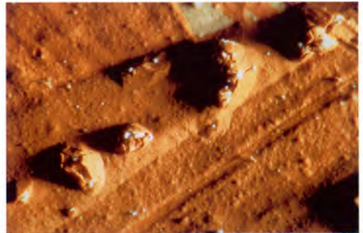
Figure 10 a/b. So-called pustules, dot-like crystallizations of salts (mostly through the formation of gypsum on the surface).
