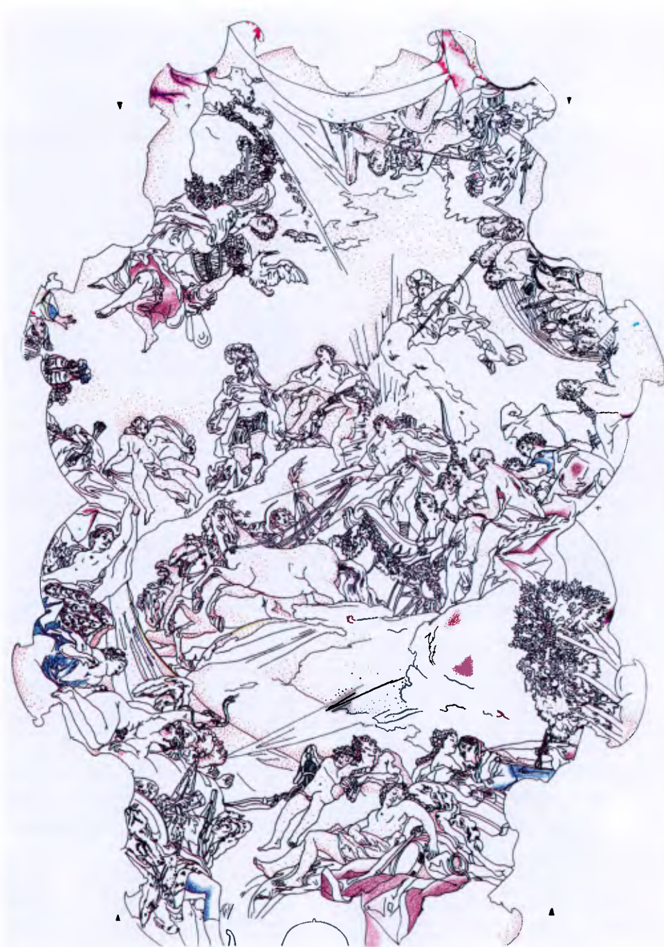
Figure 17a. Alteglöfshaus, palace, so-called “oval hall”, C. D. Asam, 1730, graphic documentation drawn after a survey photograph (see Figures 1 and 16), mapping of paint-layer damage with a coloured pencil.
