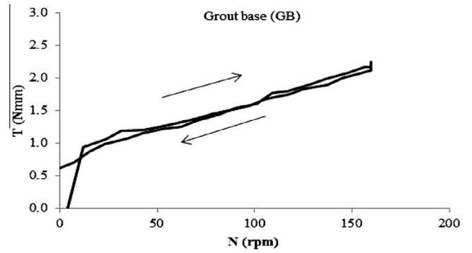
Fig. 7. Flow curves of base grout mortar (GB). The arrows indicate the up and down speed variation (GB-grout base, lime:aggregate: 1:6.6, 65 (w:w)).
