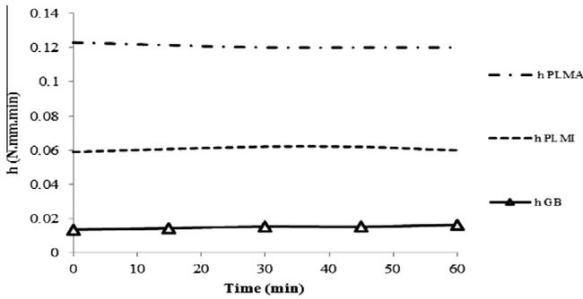
Fig. 8. Variation of  $h$  parameter as a function of testing time for the base and commercial grouts ( $h_{GB}$  – viscosity of grout base;  $h_{PMLA}$  – viscosity of grout commercial PMLA and  $h_{PMLI}$  – viscosity of grout commercial PMLI).
