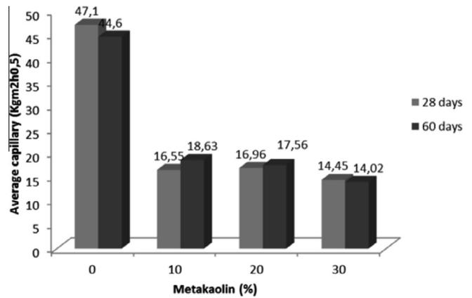
Fig. 16. Shows the effect of increasing content of metakaolin in capillarity coefficient.
