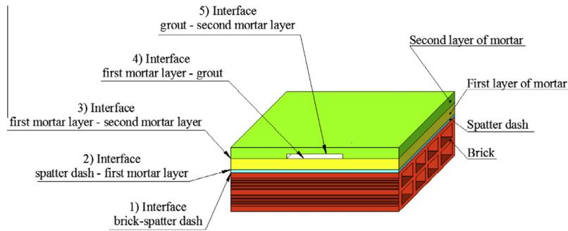
Fig. 17. Adhesion simulation sample test scheme.
