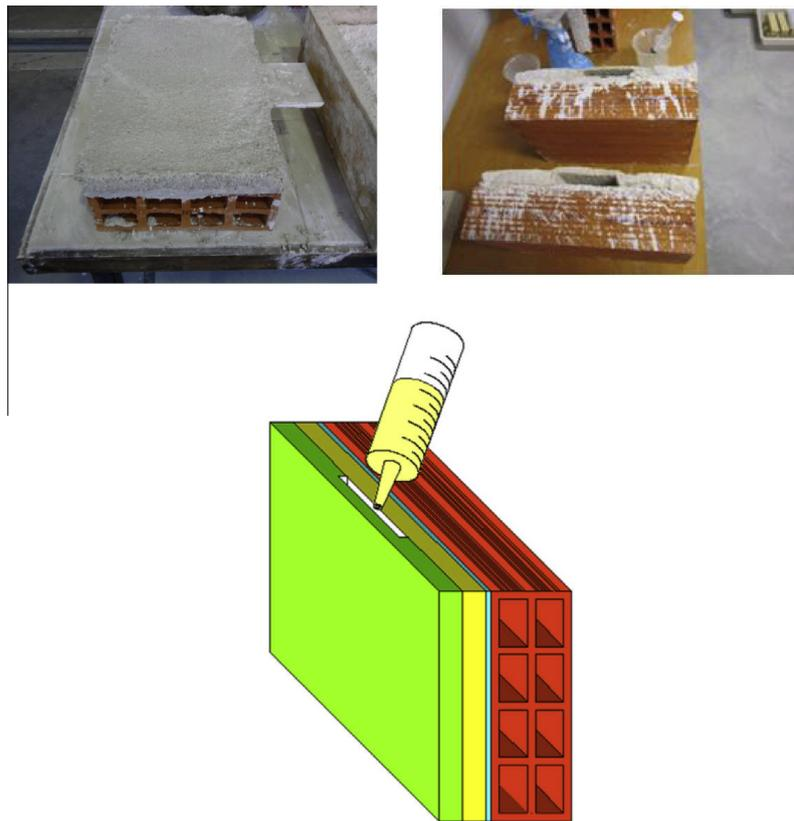
Fig. 5. Specimens simulating the detachment between layers, where the grout will be introduced.
