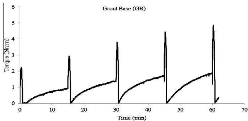
Fig. 6. Torque variation for a base grout (GB-grout base, lime:aggregate: 1:6.6, 65 (w:w)).
