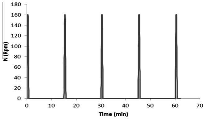
Fig. 4. Speed variation for a base grout base (GB-grout base, lime:aggregate: 1:6.6, 65 (w:w)).
