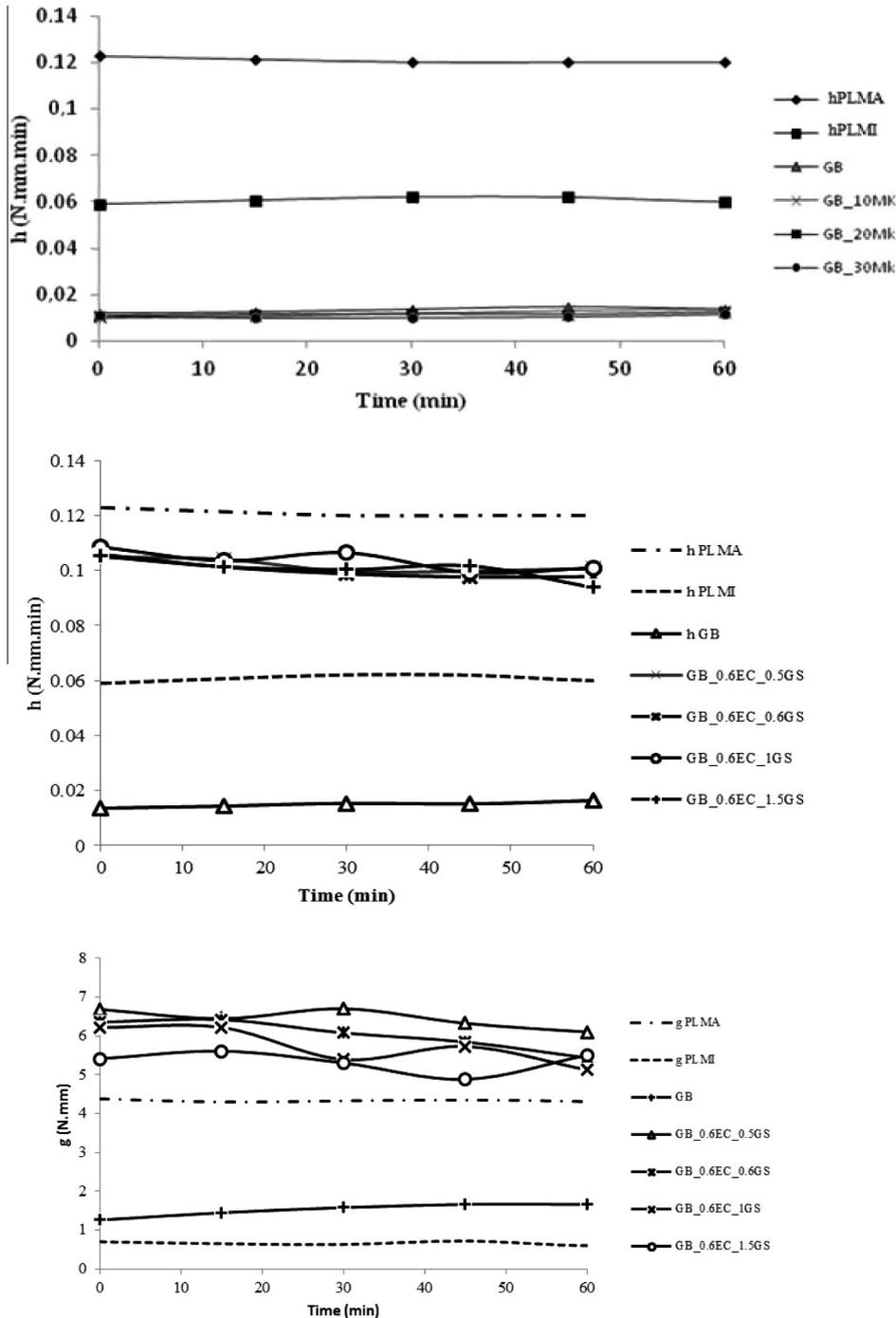
Fig. 11. Shows the effect of increasing of plasticizer agent on *h* and *g* respectively (GB\_X EC\_YGS, where X = 0.1%; 0.15%; 0.5%; 0.6% and 0.75% cellulose ether (EC) and Y = 0.5%; 0.6%; 1% and 1.5% sodium gluconate (GS)).
