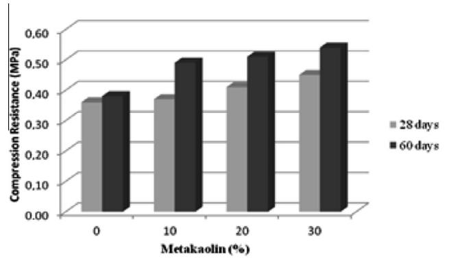
Fig. 15. Shows the effect of increasing content of metakaolin in compressive strength.
