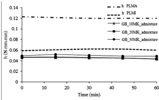
Fig. 13. Effect on h and g of increasing metakaolin content (10, 20, 30%), in grouts with admixtures (GB\_Y MK\_admixture – where Y is 10%, 20%, 30% Metakaolin, and admixture = 0.5% cellulose ether, 1% sodium gluconate and 0.5% Acril 33).
