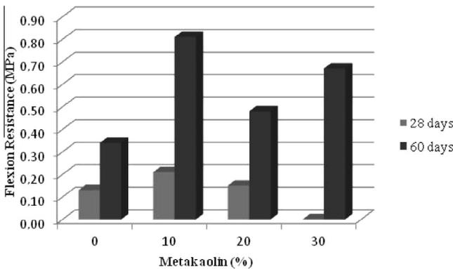
Fig. 14. Shows the effect of increasing content of metakaolin in flexural strength.
