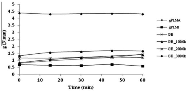
Fig. 12. Shows the effect of increasing of metakaolin (10%, 20%, 30%) on h and g, respectively (GB\_YMK where Y is 10%, 20% and 30% de Metakaolin).
