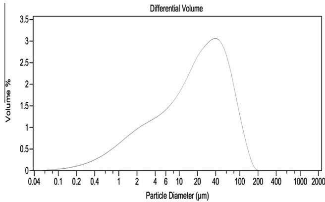
Fig. 1. Particle size distribution of silica powder.
