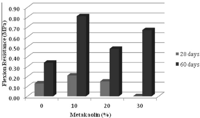
Fig. 14. Shows the effect of increasing content of metakaolin in flexural strength.
