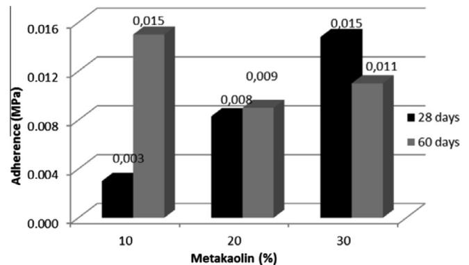
Fig. 19. Show the effect of increasing content of metakaolin in adhesion values.
