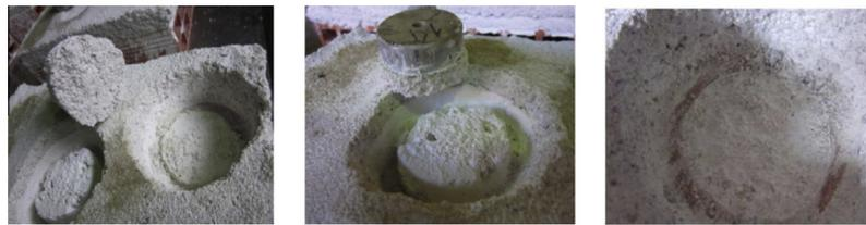
Fig. 18. Adhesion on grout and render in the samples of simulation of detachment.
