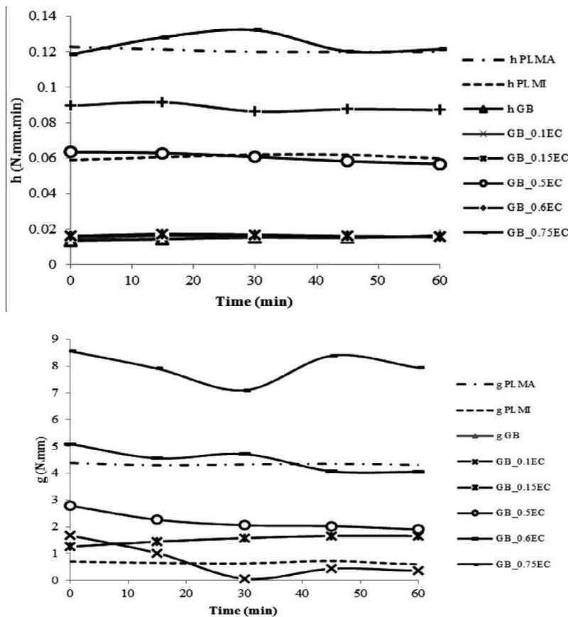
Fig. 10. Shows the effect of increasing of plasticizer agent on  $h$  and  $g$  respectively ( $GB_X EC$ , where  $X = 0.1\%$ ;  $0.15\%$ ;  $0.5\%$ ;  $0.6\%$  and  $0.75\%$  cellulose ether (EC)).
