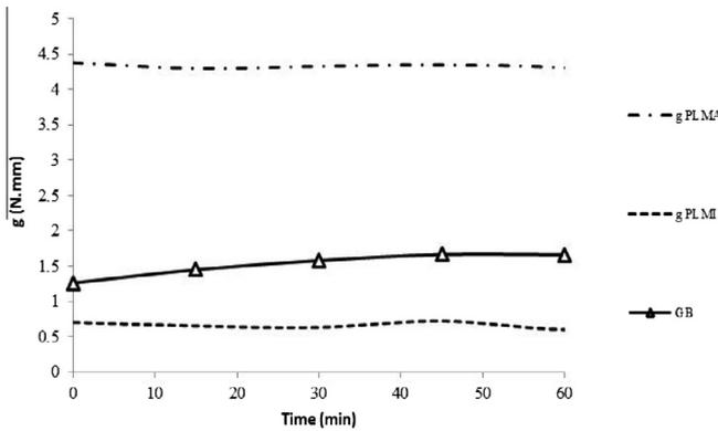
Fig. 9. Variation of  $g$  parameter as a function of testing time, for the base and commercial grouts ( $g_{GB}$  – viscosity of grout base;  $g_{PMLA}$  – viscosity of grout commercial PMLA and  $g_{PMLI}$  – viscosity of grout commercial PMLI).
