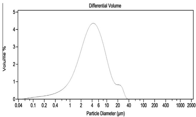
Fig. 2. Particle size distribution of metakaolin (Argical 1200).
