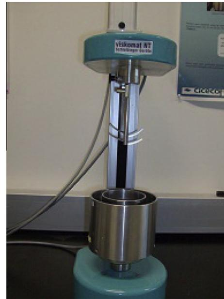
Fig. 3. The Viskomat NT rheometer measuring system.
