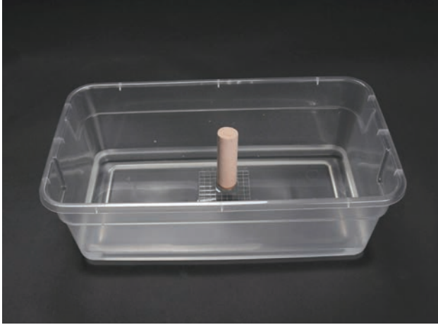
Figure 4.8.4 Specimen absorbing water after being placed in a water-filled container. The level of water absorbed is indicated by the darker area at the bottom of the grout specimen.
