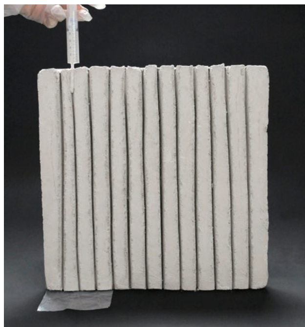
Figure 4.3.3 Injecting 10 mL grout into a channel.
