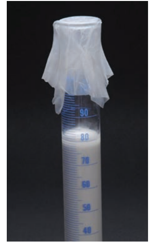
Figure 4.4.2 Bleed water at the top of the 100 mL graduated cylinder.
