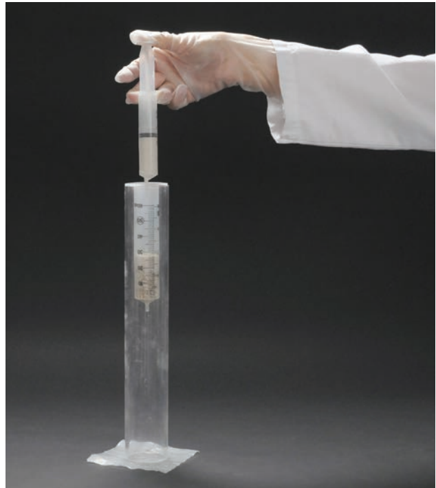
Figure 4.2.2 Injecting 20 mL grout into a 60 mL syringe. Note that the syringe with grout and granular material is held vertically and supported by a rigid plastic tube.
