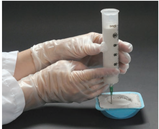
Figure 4.7.6 Syringe with cannula filled with 100 g of sand being dropped into the grout.
