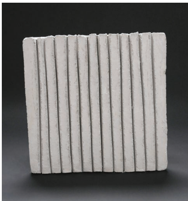
Figure 4.3.2 Prepared flow tile after setting.
