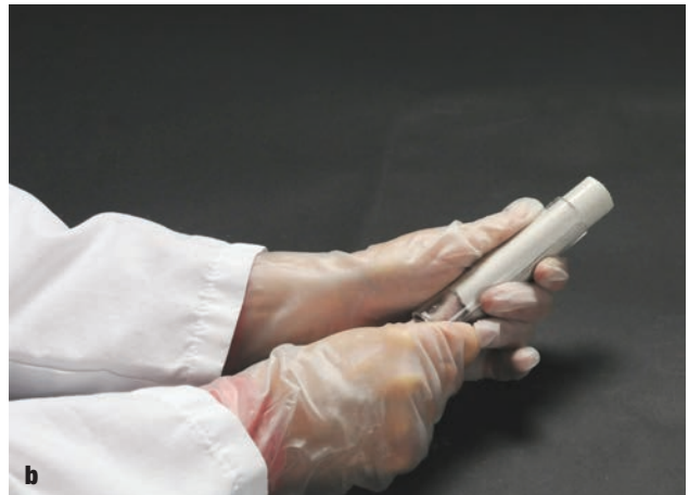
Figures 4.8.3a and 4.8.3b Slitting of a cylindrical plastic tube with a PMMA cutter (a), and removing the cured grout specimen (b).
