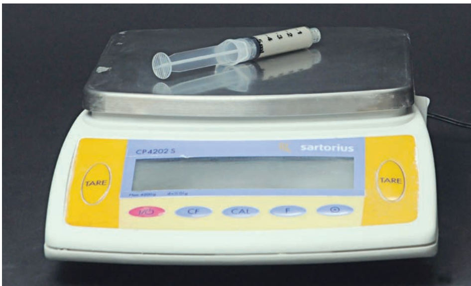
Figure 4.5.2 A grout-filled syringe is weighed.
