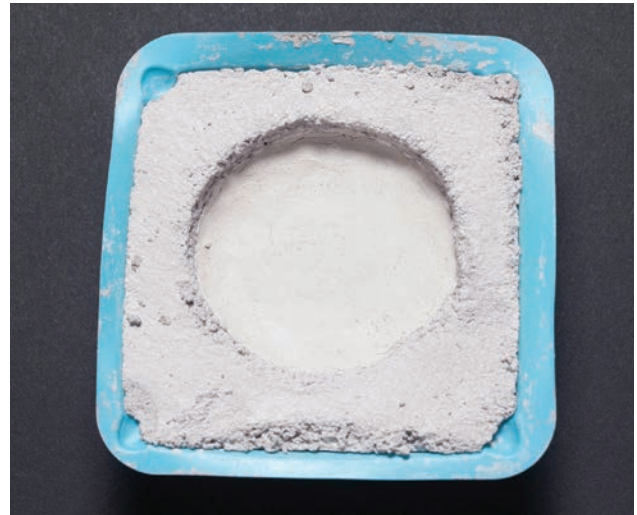
Figure 4.6.6 Specimen exhibiting no drying shrinkage (NS).
