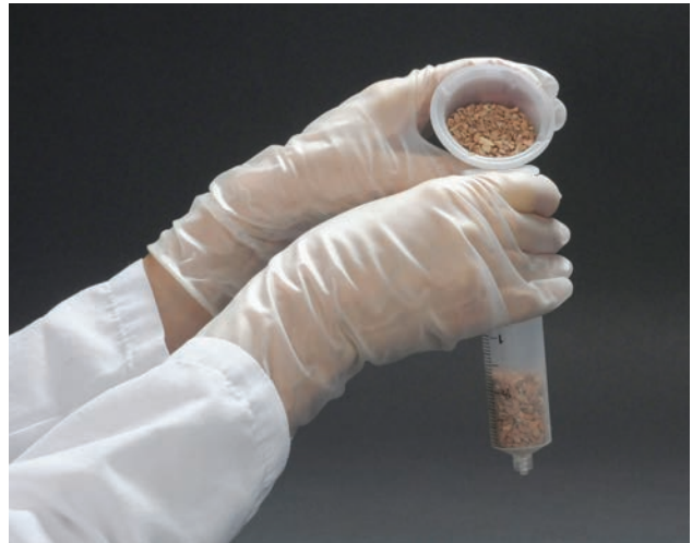
Figure 4.2.1 Pouring 20 mL crushed brick into a 60 mL syringe.
