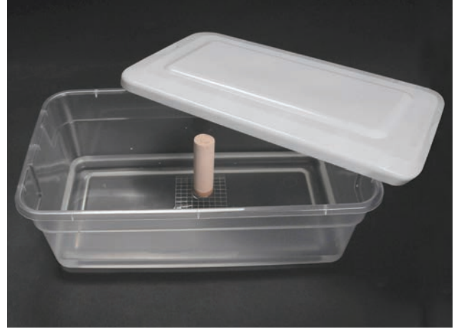
Figure 4.8.5 Test setup before covering with a lid. The cover minimizes evaporation of the water in the tray.
