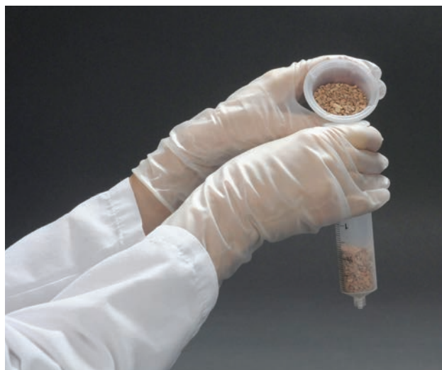
Figure 4.1.1 Pouring 20 mL crushed brick into a 60 mL syringe.
