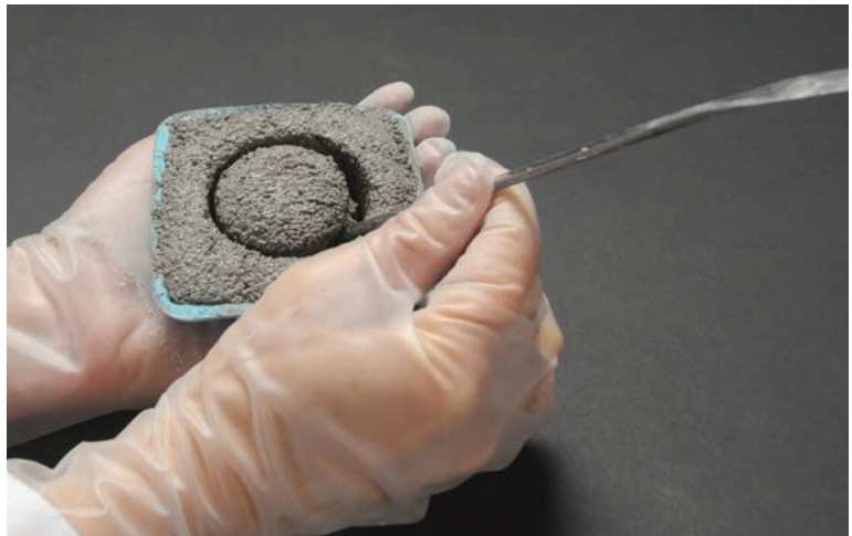
Figure 4.6.3 Removing excess mortar from the cavity.
