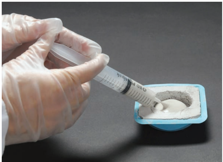
Figure 4.6.5 Grout being injected into a mortar cup.
