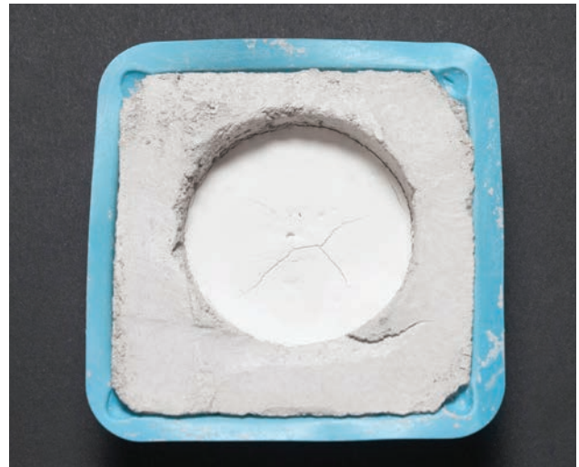
Figure 4.6.7 Specimen exhibiting medium drying shrinkage (MS).
