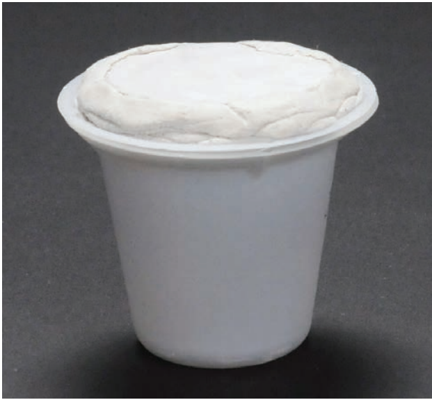
Figure 4.9.2 Cup with cured specimen after sealing.
