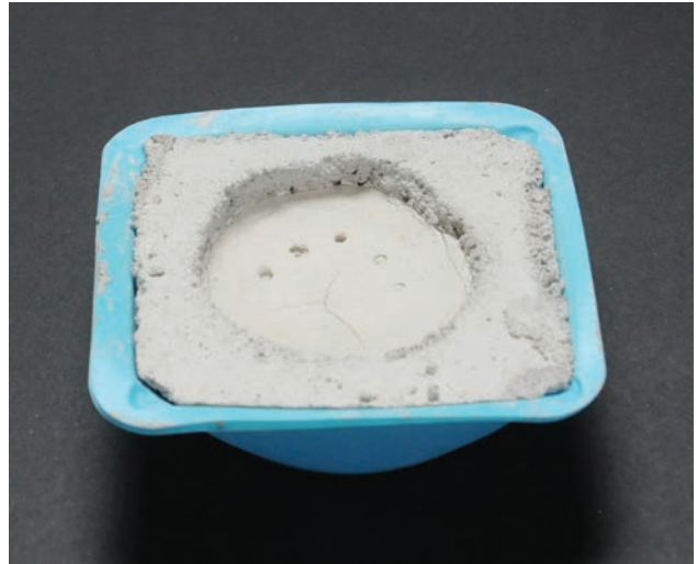
Figure 4.7.7 Final setting, reached after five penetrations.
