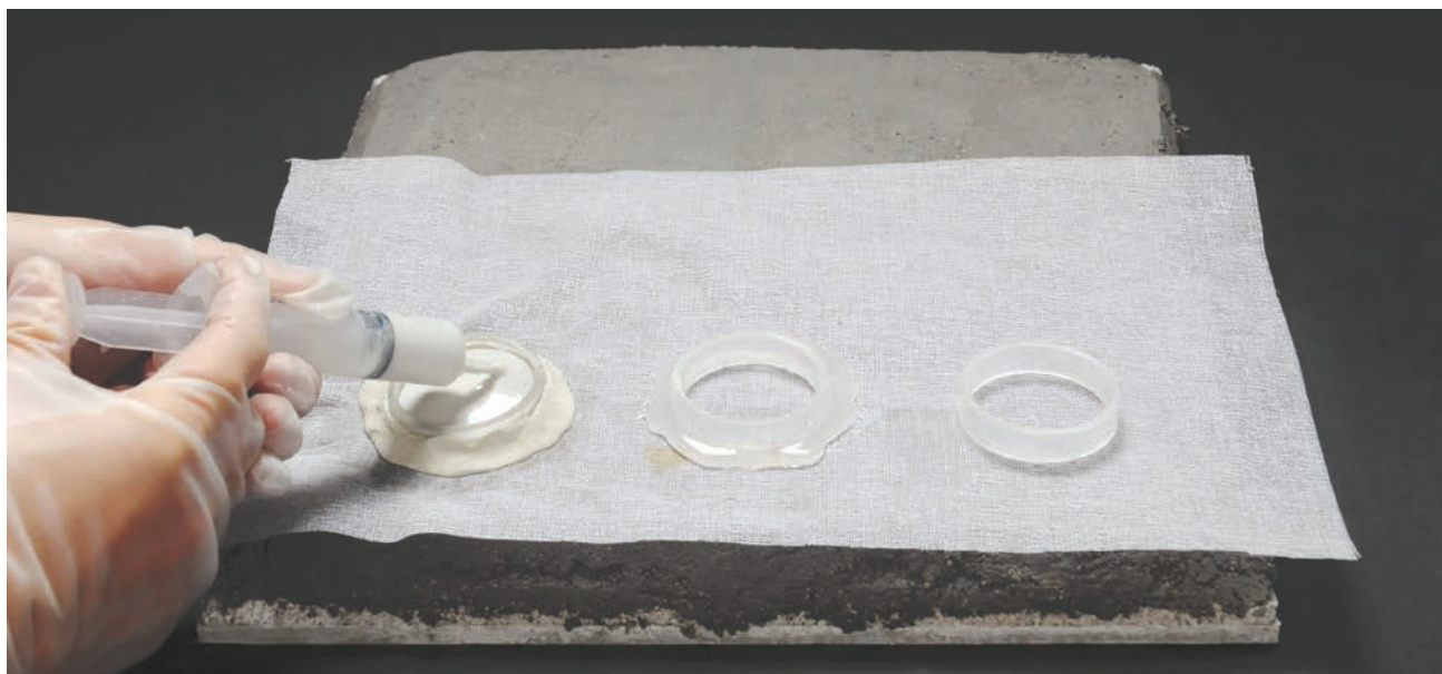
Figure 4.9.1 Molds attached to plastered tile being filled with grout.
