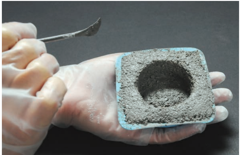
Figure 4.7.4 Fresh mortar cup.
