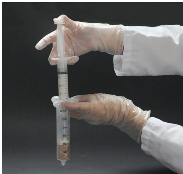
Figure 4.1.2 Injecting 20 mL grout into a 60 mL syringe.
