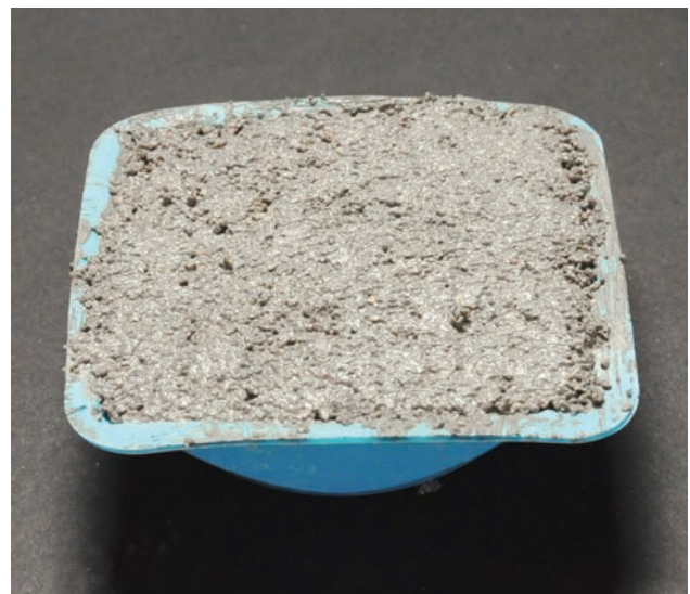
Figure 4.7.1 A weighing boat or shallow container filled with mortar.
