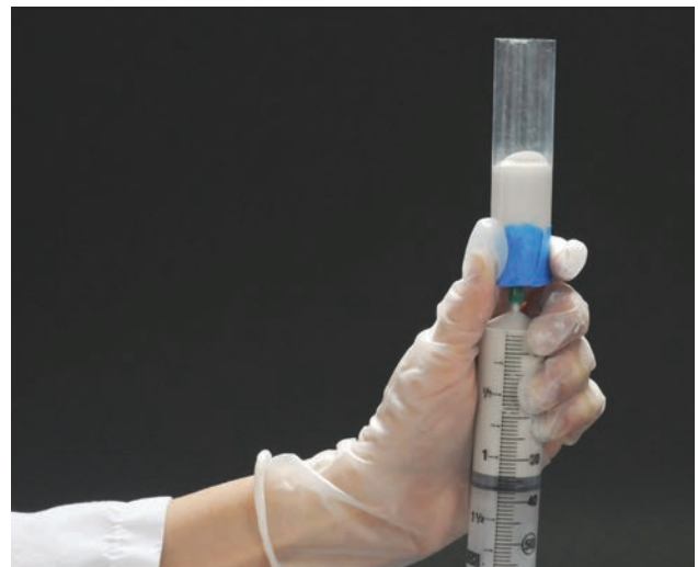
Figure 4.8.1 The column is filled with a syringe inserted from the taped bottom of the column.
